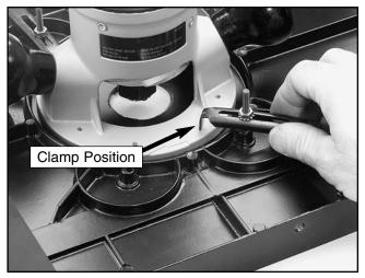
**Figure 9.** Rotating a clamp over the router base.
